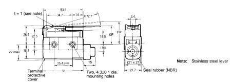
Hinge Roller Lever D4MC-2000
