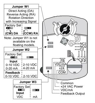
Figure 2: Calibrating the GGx Models
