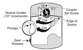
Figure 7: Switch Angle Settings
