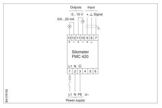
Fig. 5 Electrical connection FMC 420
