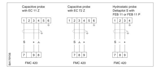
Fig. 6 Connecting probes to the Silometer (input)
