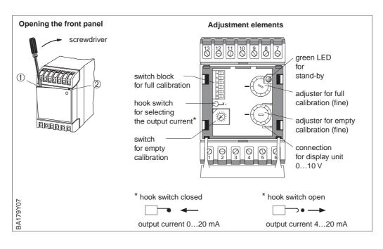
Fig. 7 Adjusting elements
