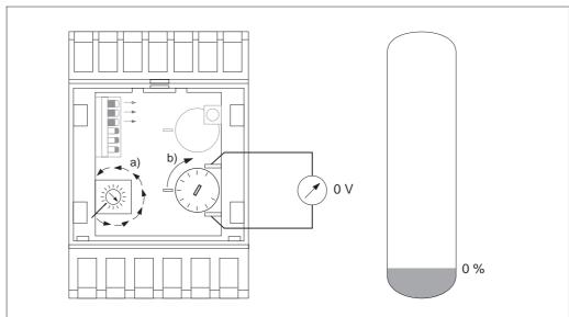
Calibration with an empty vessel
