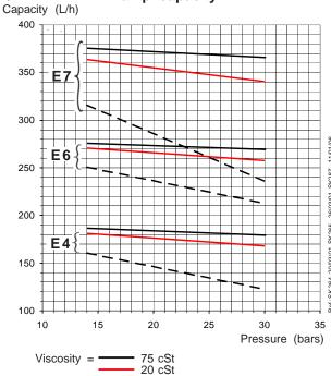
Data shown take into account a wear margin. Do not oversize the pump when selecting the gear capacity.
