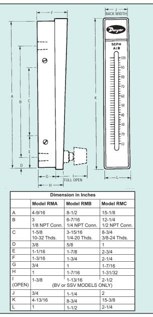
**Installation is simple** – The Rate-Master<sup>®</sup> Flowmeter can be neatly panel mounted to keep flow tube centers in the same plane as the panel surface or surface mounted on the panel by means of tapped holes in the backbone. When through-panel mounted, the bezel automatically positions the instrument at the correct depth in the panel cutout. Surface mounted units can also be held in place by the piping. All mounting hardware plus installation and operating instructions are included.
