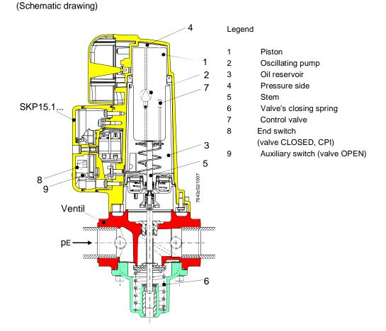
Setting 9 enabled the adaption from maximum stroke of SKP15.1... up to maximum possible stroke of combined valve.
