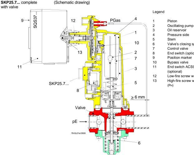
Oil reservoir Pressure side Stem Valve's closing spring Control valve End switch (optional) Position marker Bypass valve End switch ACS9.6 (optional) Low-fire screw wu (PL) High-fire screw wo
