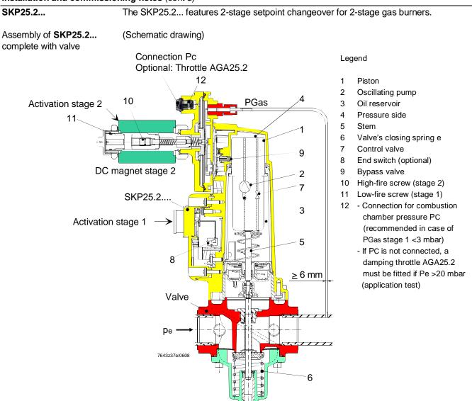
Setpoint adjustment «PGas» is made manually by turning the setting screws (10 and 11), which act on the setpoint spring.
