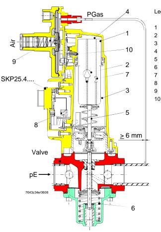
Legend1Piston2Oscillating pump3Oil reservoir4Pressure side5Stem6Valve's closing spring7Control valve8End switch (optional)9Spring (setpoint adjustment)10Bypass valve
