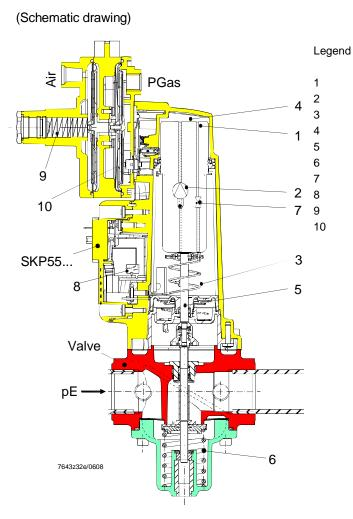
Piston Oscillating pump Oil reservoir Pressure side Stem Valve's closing spring Control valve End switch (optional) Spring (setpoint adjustment)
