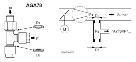
The reducing T-piece AGA78 is supplied ready for mounting, with D1 = 1.5 mm and D2 = 1.7 mm.
