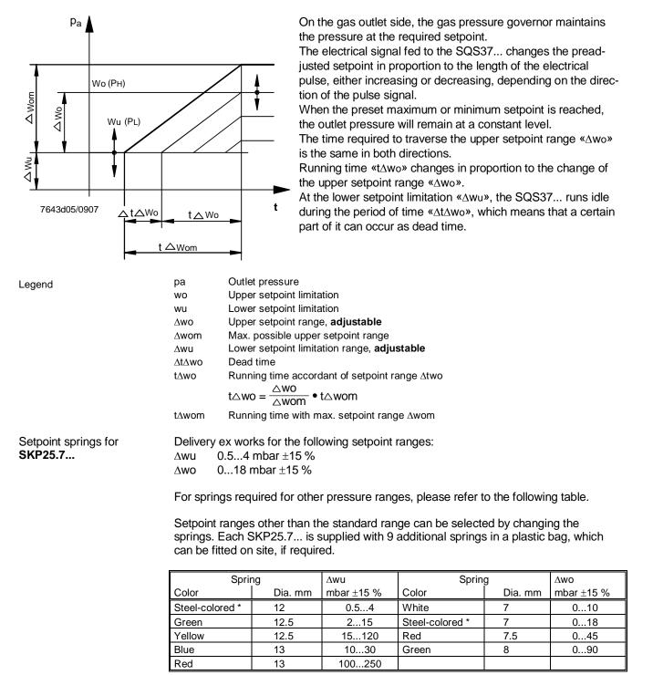
Functioning principle of gas pressure governor with SQS37... motorized setpoint adjuster:
