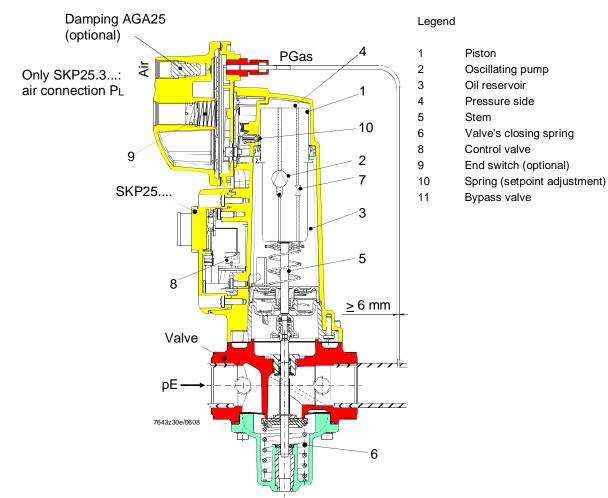
**SKP25... / SKL25...** Setpoint adjustment «PGas» is made manually by turning the setting screw, which acts on the setpoint spring (for setpoint springs, refer to «Accessories»).
