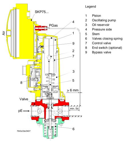
Adjustment of governor on modulating burners
