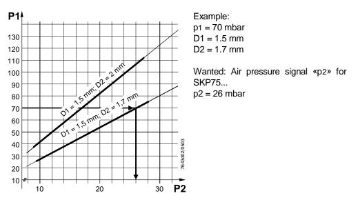
Air is continuously vented to atmosphere via orifice «D2». The pressure of the following medium will be reduced via throttle «D1». The illustration below shows the correlations.
