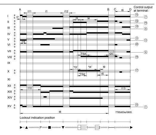
\* Times safety time (TSA'), long preignition time (t3') and interval (t4') are only programmed by burner controls LGK16.335... and LGK16.635...
