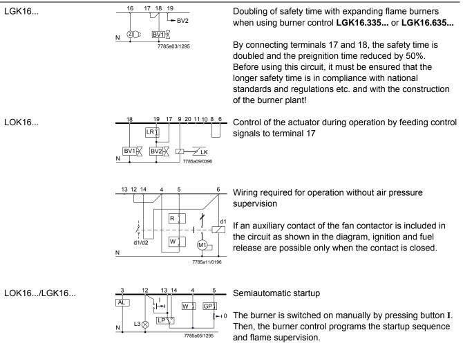
The burner is switched off manually by pressing button  $\mathbf{0}$ , or automatically by the limit thermostat or pressure switch (W), or by gas pressure switch (GP). Signal lamp (L3) indicates when the burner control is ready to be started; it extinguishes shortly after the burner is switched on.
