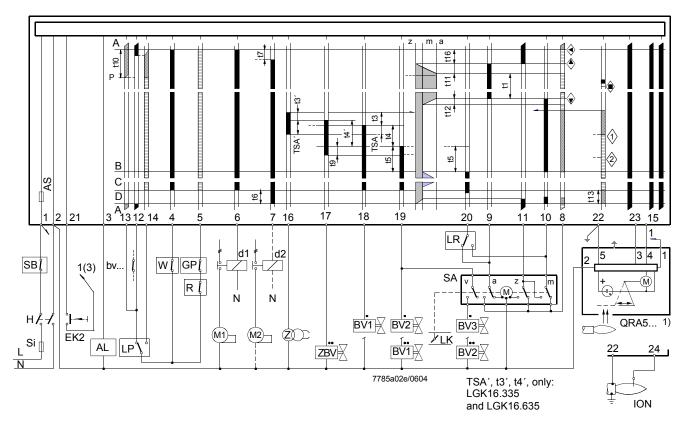
1) When used in connection with QRA53.../QRA55..., earthing of terminal 22 is mandatory!
