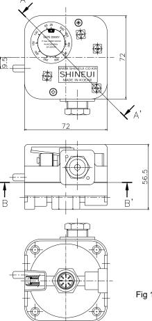
Fig 1. Gas pressure switch(V)
