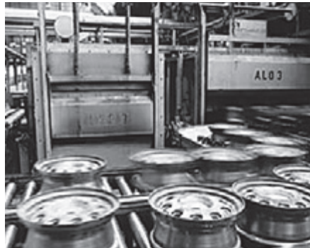
Aluminium industry: curing oven for wheel rims
