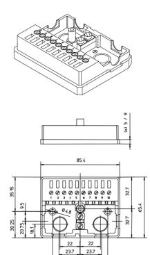
(\*) The dimensions differ depending on the type of socket: 5 with socket D 9 with socket E
