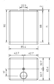
h: Dimensions depending on the type of socket: 95 with socket D 99 with socket E 98.3 with socket NE
